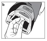
Pre-Filter with your fingers. Empty any dirt, debris, or liquid from the Bowl and Pre-Filter
